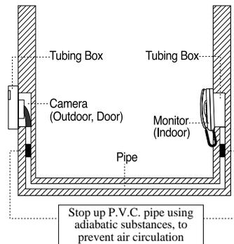
※ Stopping up pipe as above minimizes temperature difference between indoors and outdoors, and also eliminates moisture and condensation on door camera window.
