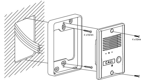
After attach the body supporter with 2 screws, put the Door Camera into the grooves of body supporter, and then fix it with 2 screws and stick the finishing materials.
